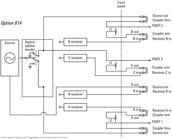
Note: Option 1E1 adds a 70-dB step attenuator between the source and the switch splitter leveler.
