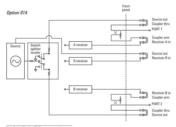
Note: Option 1E1 adds a 70-dB step attenuator between the source and the switch splitter leveler.
